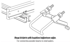
Hook strap for connecting timber beams to steel walers. For connecting wooden beams to steel walers.
